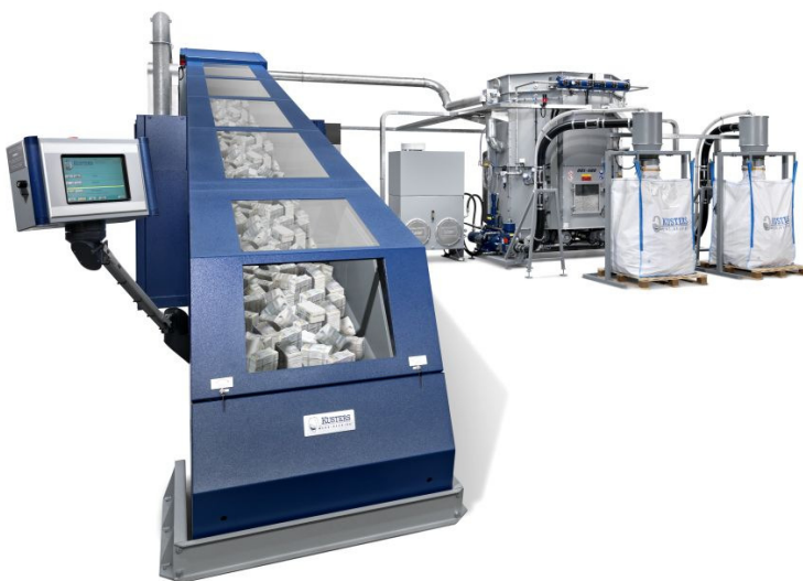
An off-line banknote destruction system
